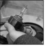
3. Pull the bulb/socket straight out from the headlamp housing.
